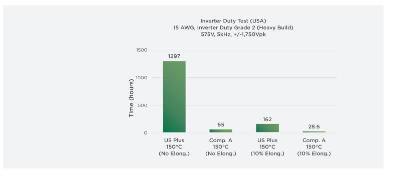
The following categories show even more of an advantage for UltraShield® Plus. It performed better than Comp. A in the Inverter Duty test (both with no elongation and with 10% elongation), Inverter Duty Withstand test, and Pulse Endurance test. The test results were especially more favorable at elevated temperatures and elongation.
